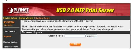
**NOTE:** Be aware that if you have started upgrading firmware, please DO NOT turn the MFP Server off. That will make the MFP Server damage due to the firmware doesn't upload complete.
